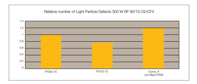
The above chart shows the relative particle generation of three material technologies:
