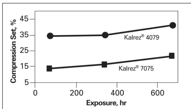
Figure 1. Compression Set at 204 °C
